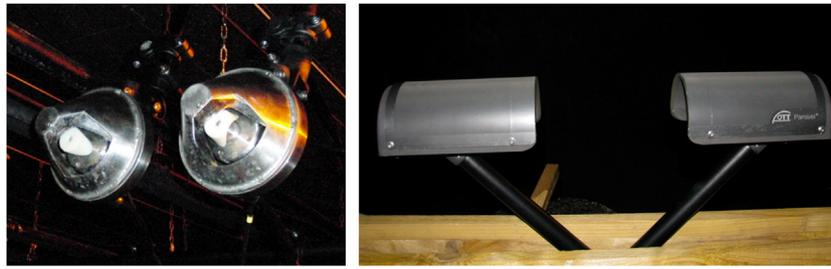
Fig. 1. The two sprayers of the rain simulation system (left) and the spectro-pluviometer (right).
